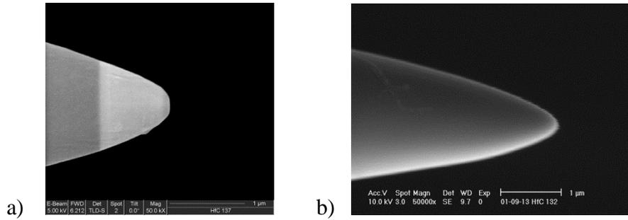
Figure 1: Micrographs of HfC(310) tips a) #137 and b) #132.
